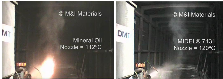
Figure 4: Image from the Spray Ignition Test (a) Mineral Oil & (b) Synthetic Ester
