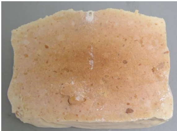
Figure 7: Post-test sample after the 100 mm basket test at 65°C
