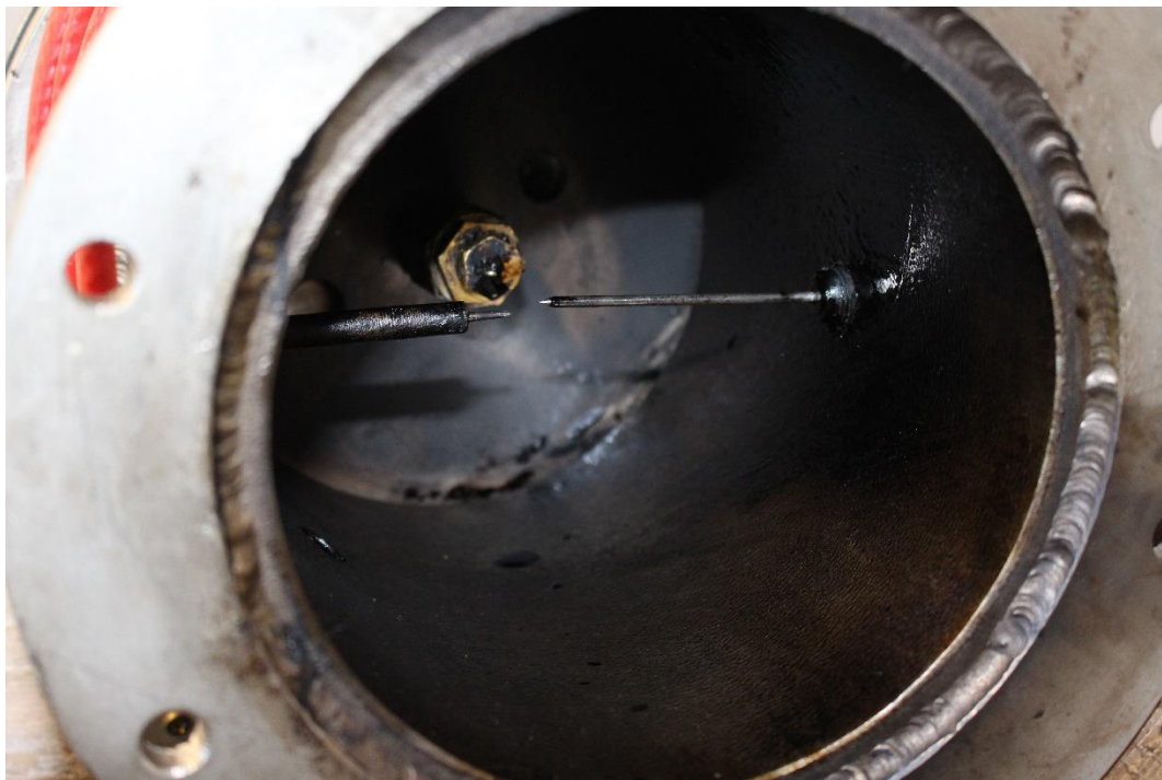
Figure 3 - Oil Mist Flammability Test Setup - Closed Vessel (Internal)
