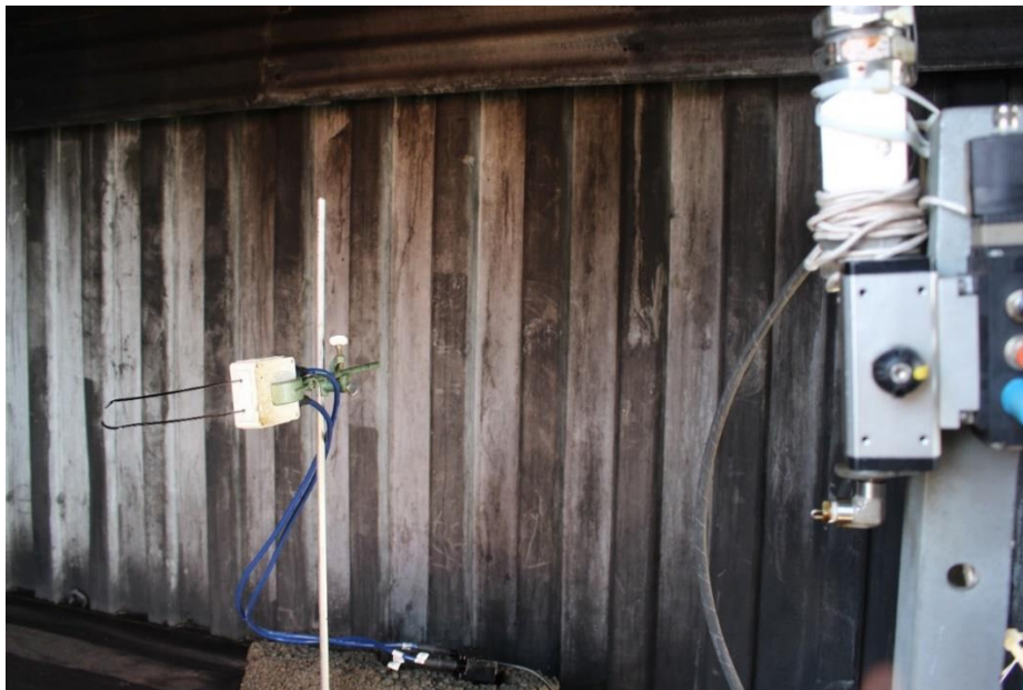
Figure 5 - Oil Mist Flammability Test Setup - Open Jet - side view
