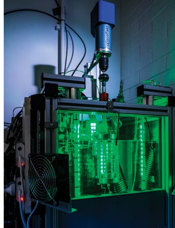
The high pressure sapphire visual autoclave is used to study hydrate plug formation and characterise crude oils. PHOTO: MATTHEW GALLIGAN/UWA
