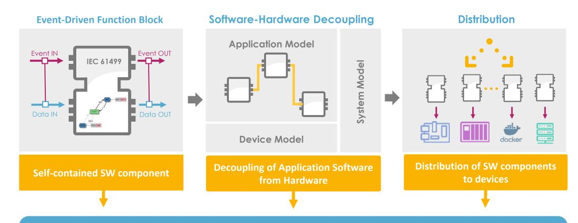
"Plug & Produce programming using hardware-independent, proven-in-use libraries of software components"
