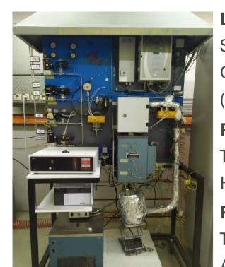
**Loading** reactor with mixture: Sorbent:  $66wt\%CaO/CaZrO_3$ OC:  $40wt\%Ni_XCo_{(1-X)}O/ZrO_2$ ( $Ni_XCo_{(1-X)}O)/CaO = 0.5$
