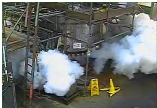
Figure 1: Discharge of White Dust from the Filter Dryer Gasket
