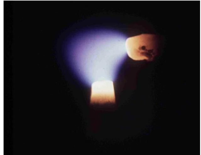
View of arc, 10-15 A in nitrogen
