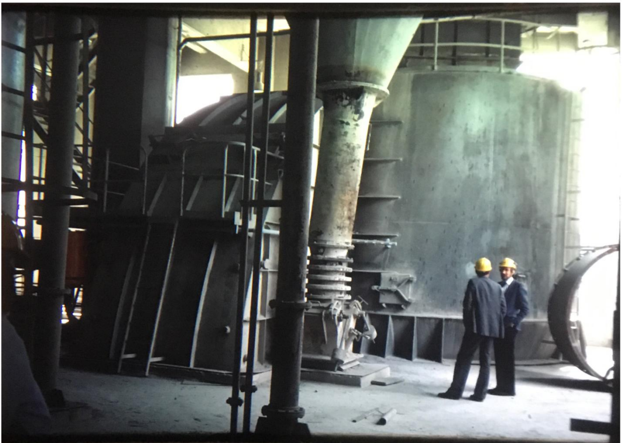
The collection valve of a cyclone, with blower, cement works, UK
