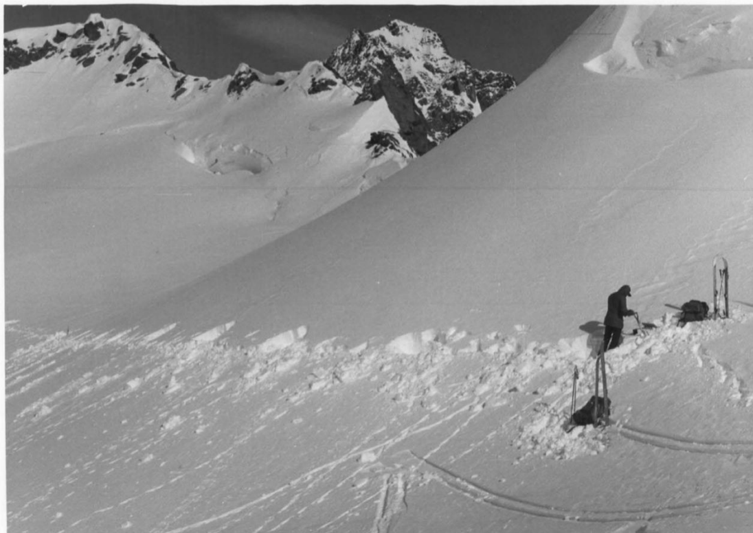
Plate 5 : Multiple pits across the Murchison Headwall to measure spatial characteristics of strength.
