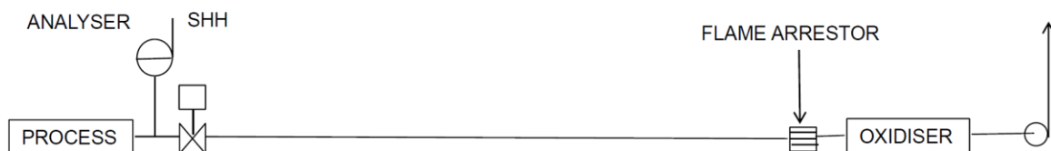
Figure 9 Simplified diagram to show means of prevention of blow-back
