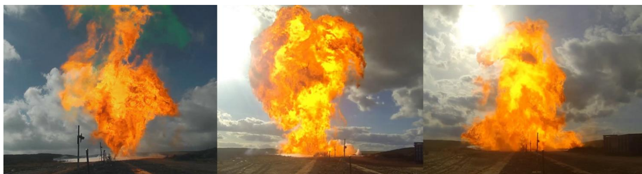
Figure 4: Induced LNG BLEVEs three seconds after rupture of the 5 m 3 vessels; Left - Experiment 2 (37% fill, 13 barg), Middle - experiment 3 (67% fill, 6 barg), Right - experiment 4 (69% fill, 13.6 barg).
