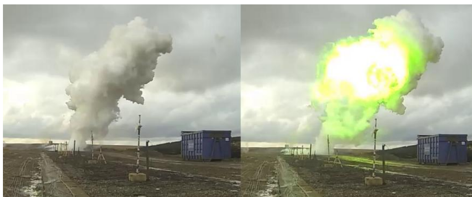
Figure 3: The induced LNG BLEVE in experiment 1, showing the resultant flashing cloud (left) and fireball (right) approximately 3 seconds after rupture
