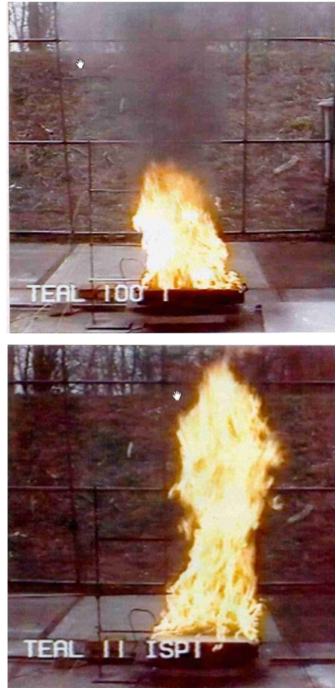
Figure 5: Flame height of a 1 m 2 pool fire of neat TEAL and 11% TEAL / isopentane solution; Source AkzoNobel 5
