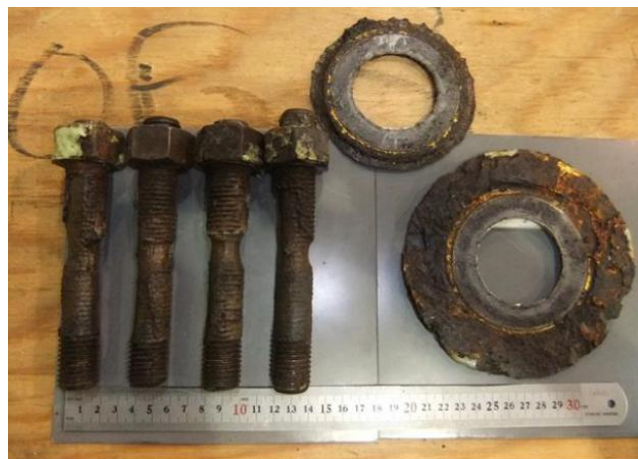
Figure 11: The situation in Figure 10 was much worse when the bolts were removed. The bolts had lost up to 35% of their thickness!
