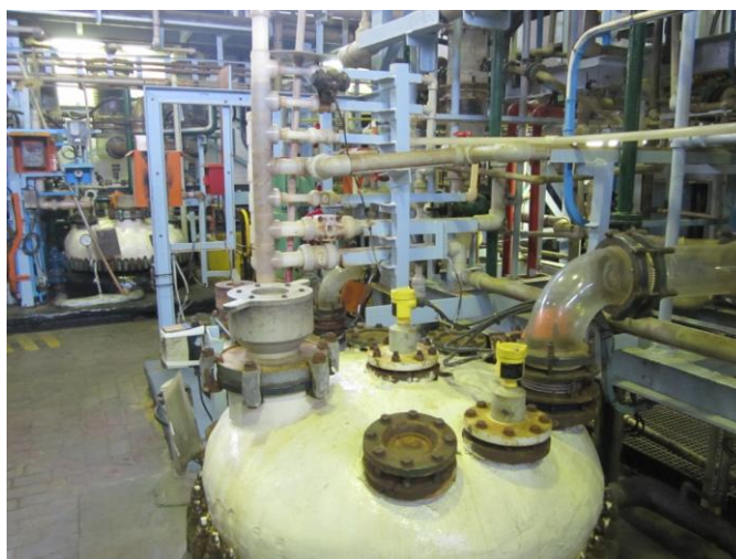
Figure 7: Ruthenium reactor – only one of the three reactors allowed water addition – inconsistency
