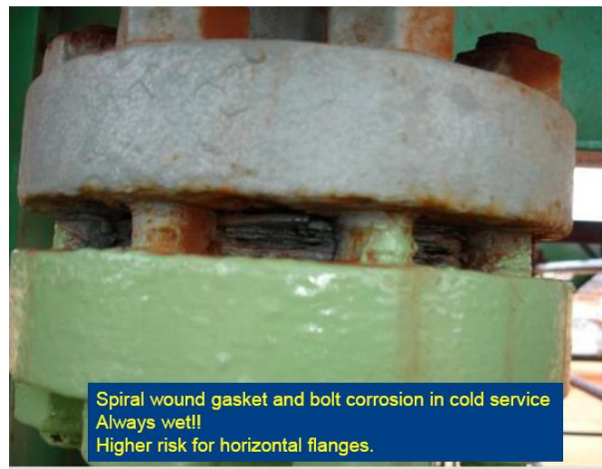
Figure 10: Cold service often produces wet conditions for flange bolts. Corrosion risk for horizontal flanges and bolts
