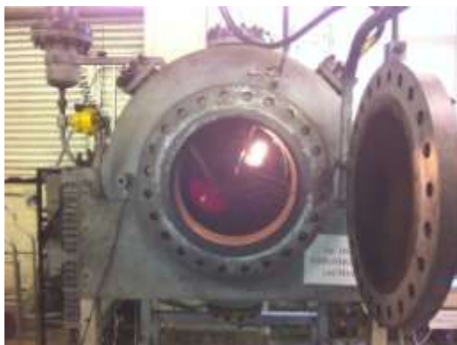
Figure 1 The University of Leeds modified 1m 3 explosion test vessel
