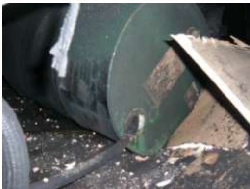
Figure 10: DECC drum with reactor feed line inserted
