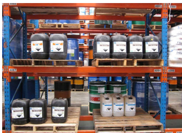
Figure 2. Picture 2-Warehouse – oxidizers/acids adjacent & overhead
