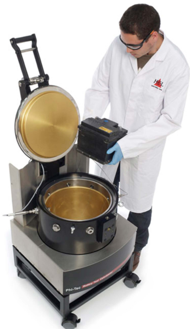
Figure 4. Custom designed Battery Testing Calorimeter (BTC) for larger scale testing
