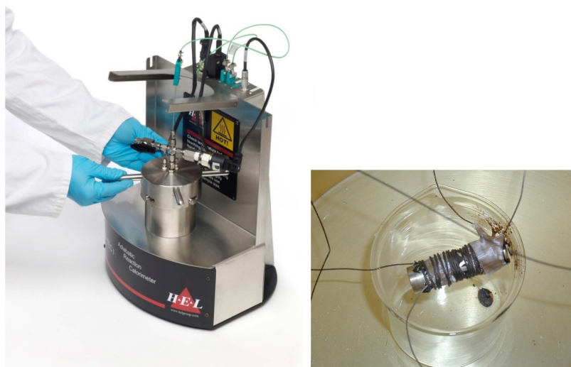
Figure 3. Phi-tec I - standard "ARC-type" adiabatic calorimeter for small scale thermal stability testing. An 18650 battery shown after test is such a unit
