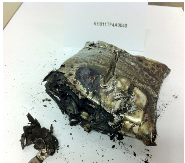
Figure 12. Li-ion Battery after overcharging test in BTC
