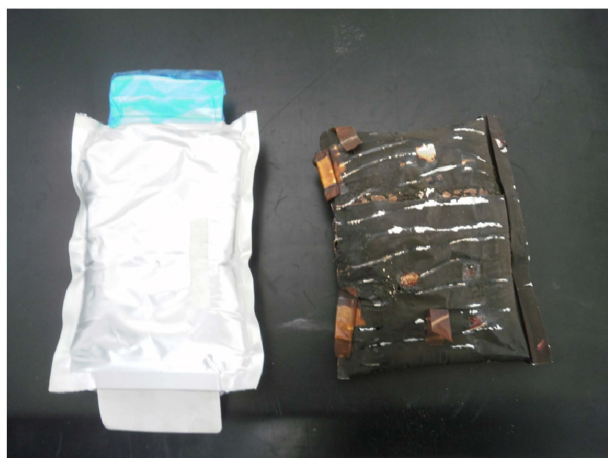
Figure 6. Pouch battery before and after heat-wait-search Test
