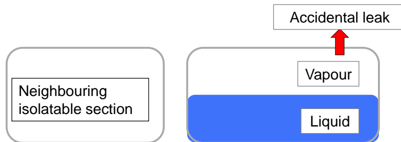
(c) following successful isolation and before blowdown ( t_{ESD} < t < t_{BD} )
