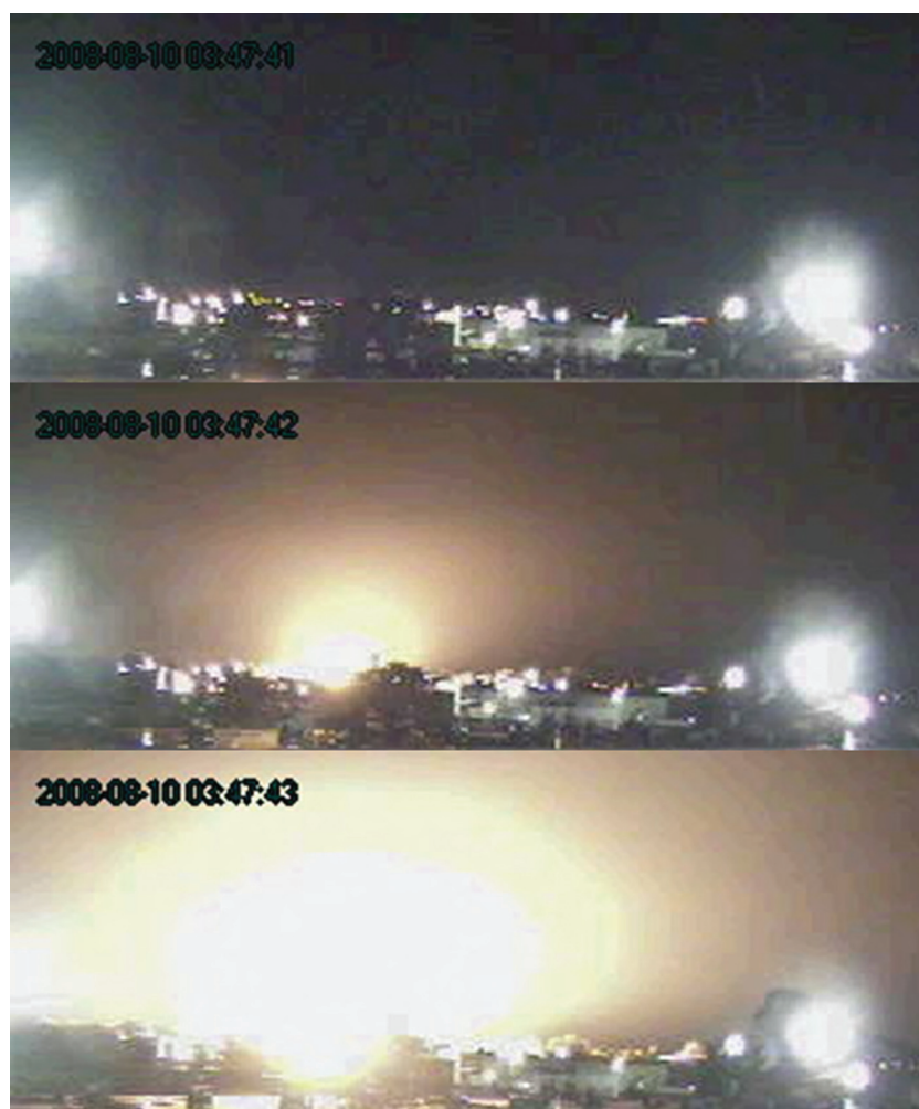
Figure 1. Three frames from a CCTV camera observing Sunrise Propane explosion from a distance. The very fast flame acceleration into the third picture ( > 1000 m/s), a very intense light, as well as videos captured from other angles seeing flames accelerate through vegetation were among the reasons for concluding a DDT was seen (Ontario Fire Marshal, 2010). Courtesy of Ontario Fire Marshals Office.
