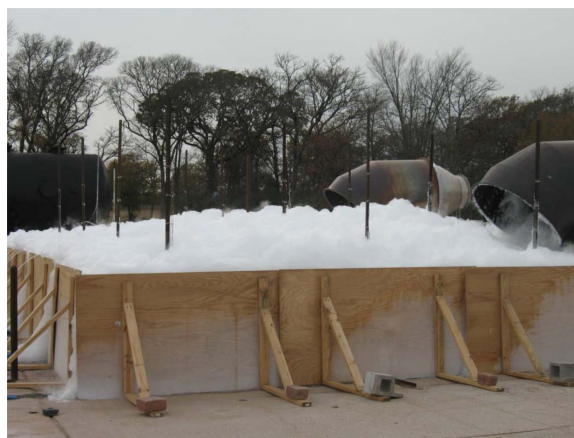
Figure 7. Expansion foam application on LNG vapor dispersion (Yun 2011)
