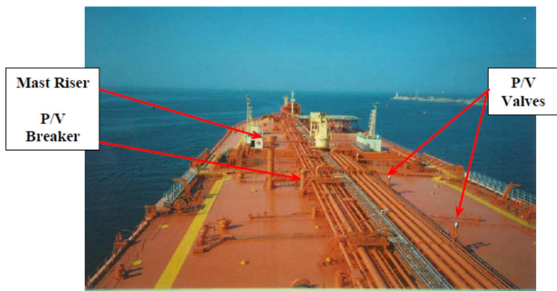
Figure 3. Typical deck layout of a very large crude oil carrier
