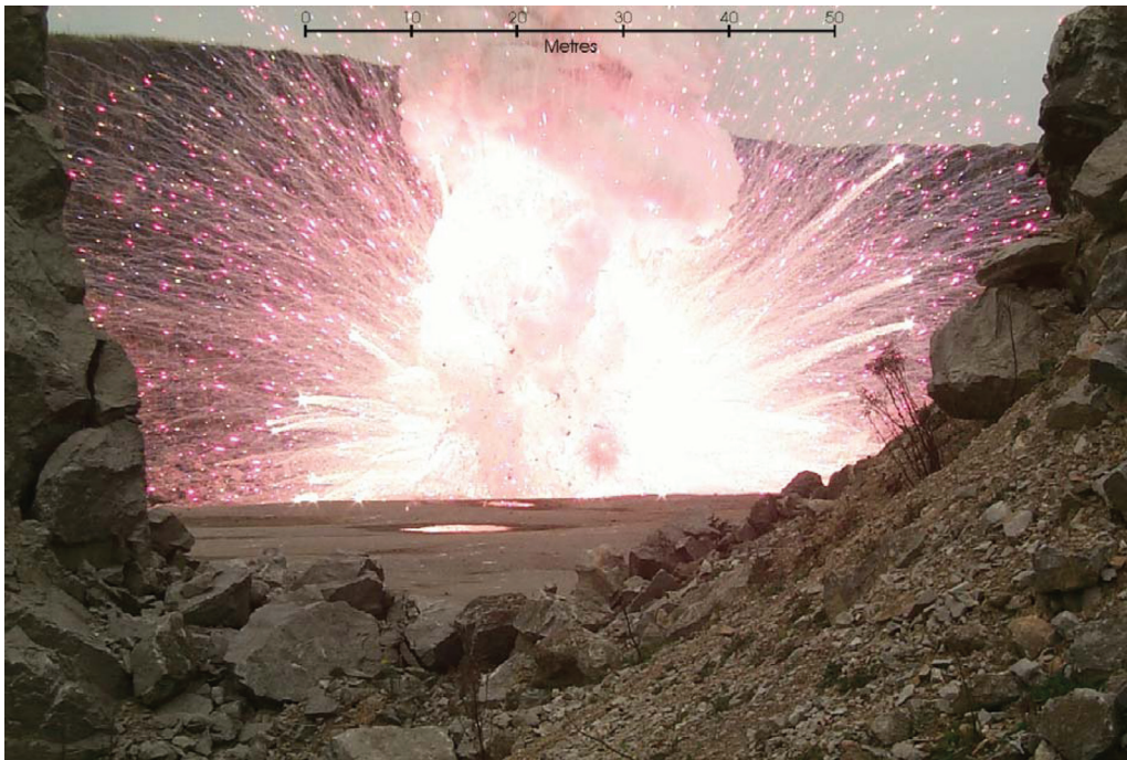
Figure 3. Effects of ignition of 2.6 tonnes NEC of firework shells in a 20 ft steel ISO transport container
