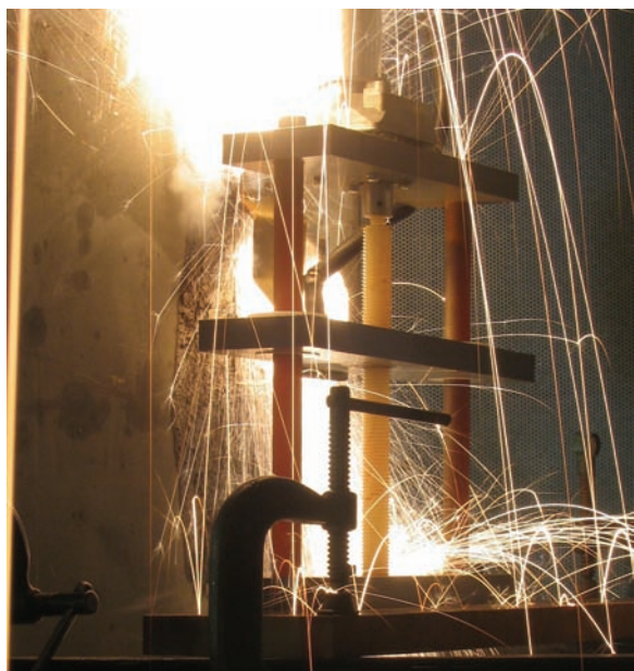
Figure 6. Test result for conduction of Long Duration Currents only, at 800 A for 5 ms
