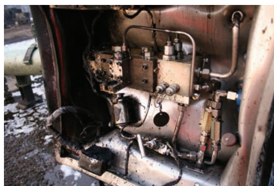
Figure 4. Steel enclosure crushed by a SVCE – minimal shape recovery
