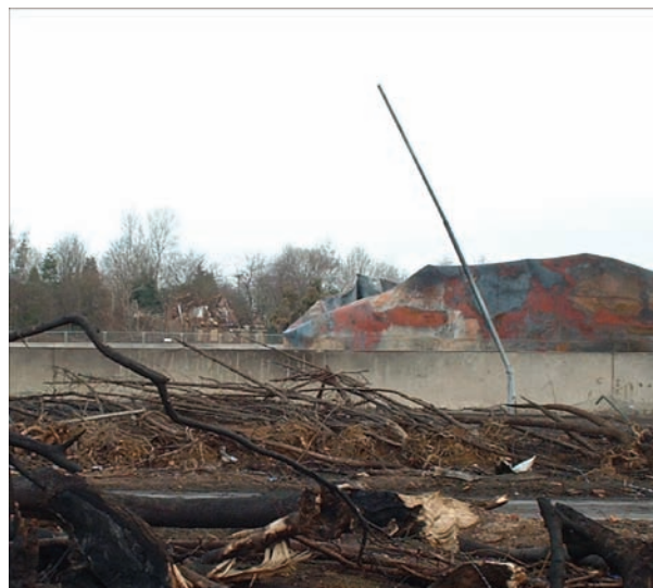
Figure 13. Posts and trees deformed by drag forces in the explosion
