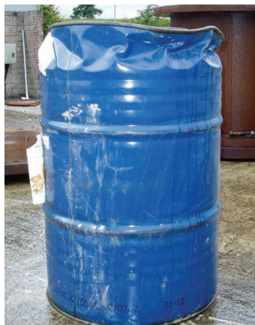
Figure 5. Crushing of drum wall in the ullage – not seen below 200 kPa
