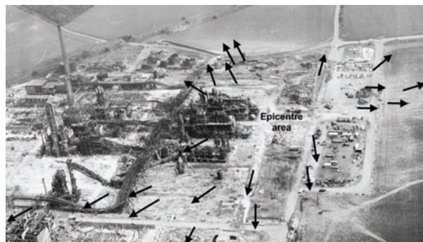
Figure 12. Directional indicators (net drag) at the Flixborough incident
