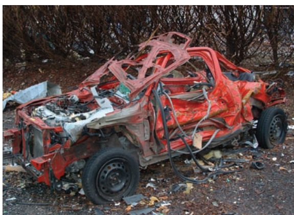
Figure 1. Car crushed by a severe VCE without overturning
