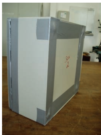
Figure 7. Two views of damage to box (300 × 300 × 150 mm) caused by 100 kPa (1000 mbar) overpressure (static test): slight bowing of back but no plastic deformation of front
