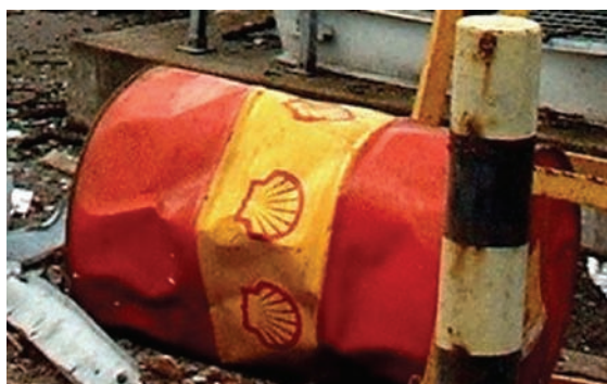
Figure 3. Drum crushed in a SVCE but showing near complete volume recovery
