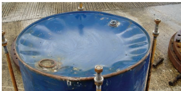
Figure 6. Plastic deformation of drum end cap – not seen below 200 kPa
