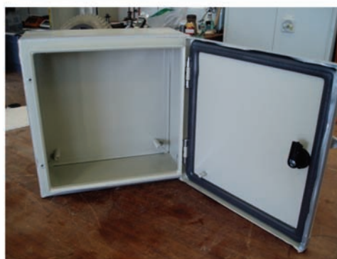
Figure 7. Two views of damage to box (300 × 300 × 150 mm) caused by 100 kPa (1000 mbar) overpressure (static test): slight bowing of back but no plastic deformation of front
