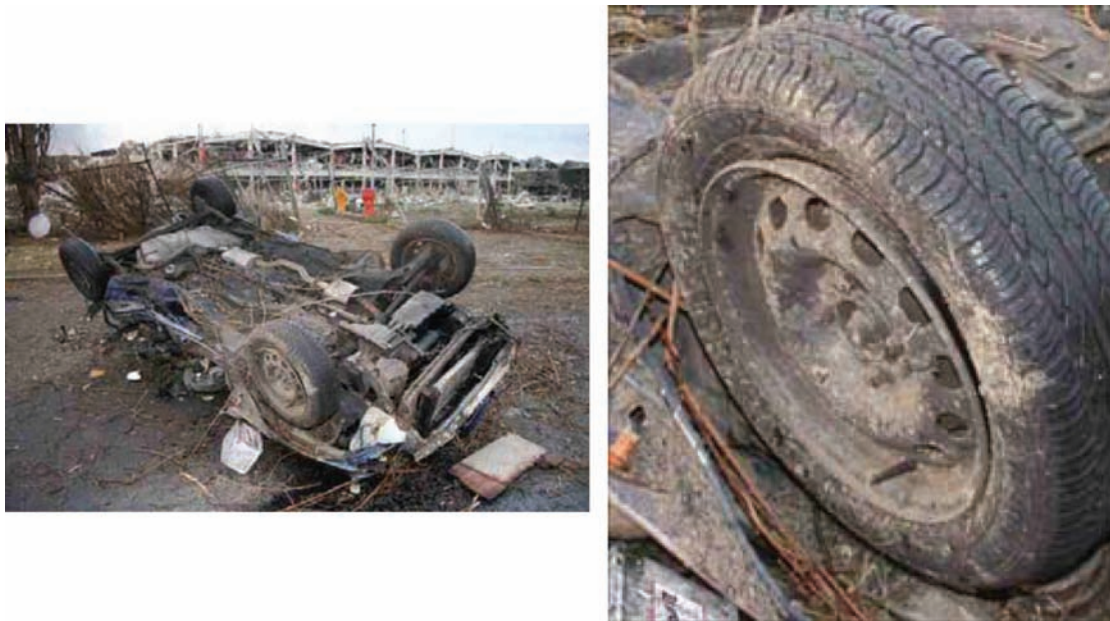
Figure 8. Tyre pushed off inner rim during explosion
