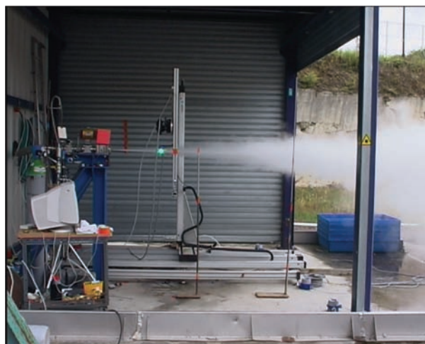
Figure 6. PDA droplet size measurement for large-scale butane jet experiment (INERIS)
