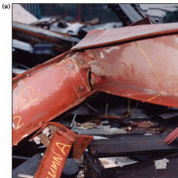
Figure 8. (a,b) Showing the damaged steel I section structure with characteristic detachment of supporting leg, bottom right
