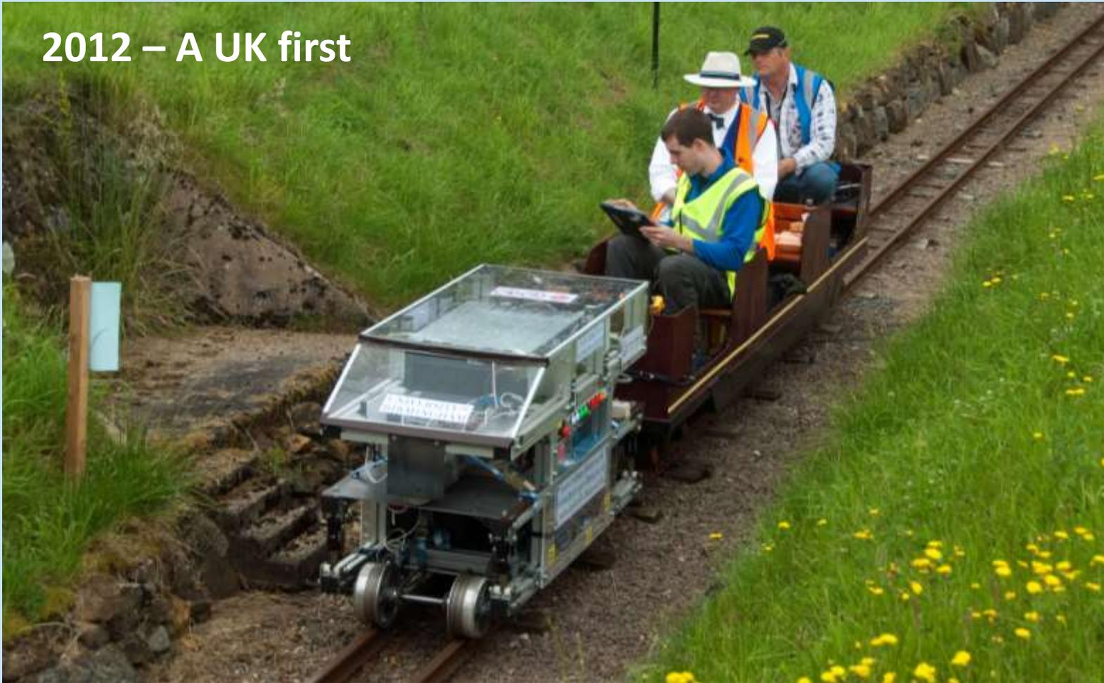
University of Birmingham's Hydrogen locomotive powered by a 1kW fuel cell at the IMechE's Railway Challenge on the Stapleford 10 ¼ inch miniature railway 1<sup>st</sup> July 2012
