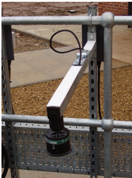
Picture 5. Ultrasonic sensor with hinge
