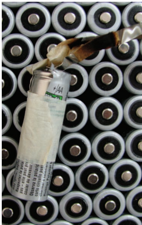
Figure 4. Packaged batteries with hard shorted cell showing paper charring
