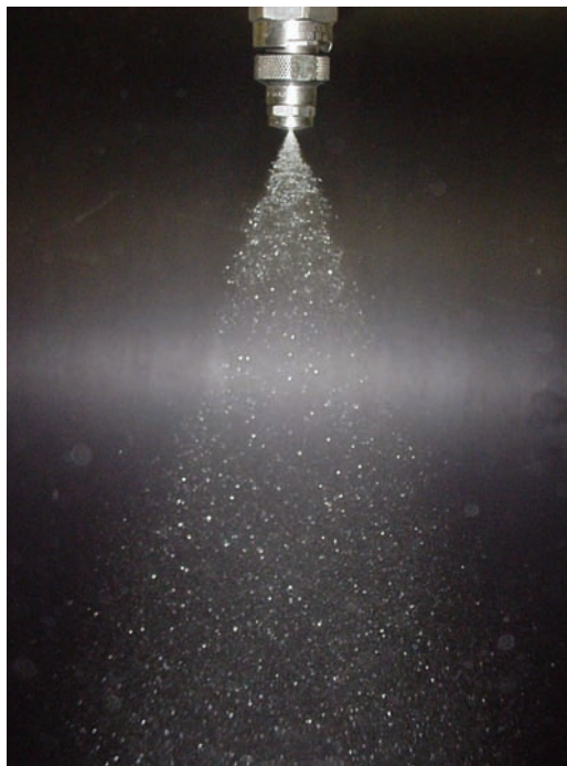
Figure 1. Single fluid nozzle
