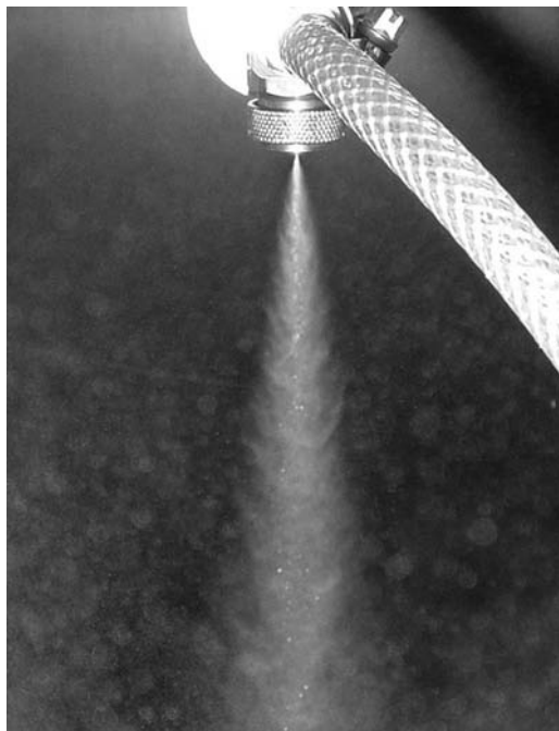
Figure 2. Twin fluid nozzle
