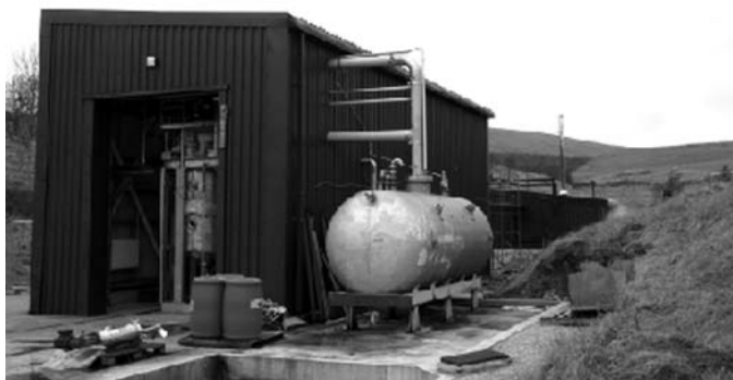
Figure 5. Large-scale facility for investigating runaway reactions
