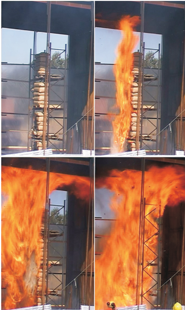
Figure 3. Rapid fire growth in wood dust Times from ignition: Top left: 11 min 30 s Top right 11:45 Lower left 11:50 Lower right 11:55
