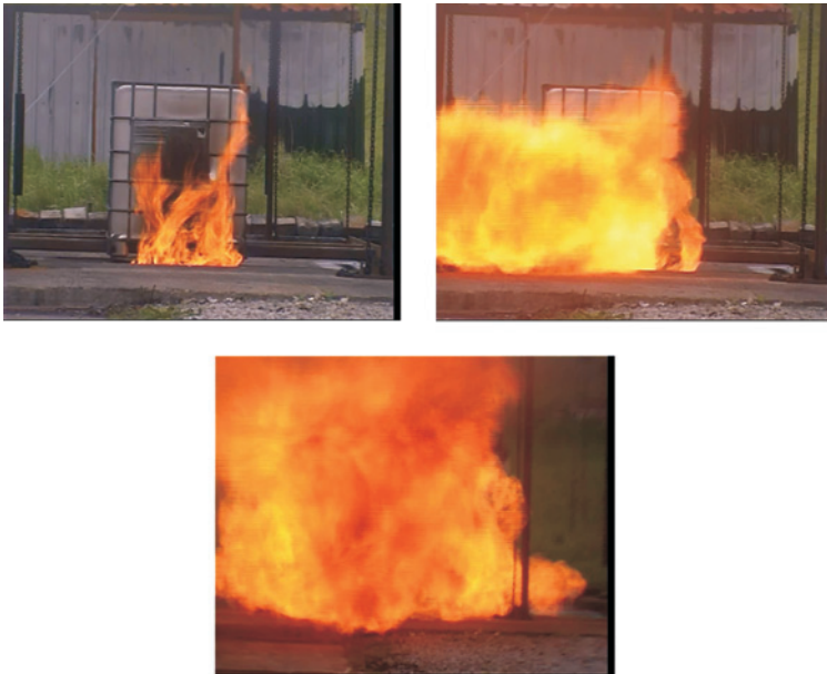
Figure 6. Consequences of ignition of IPA vapour in the ullage of a part-full IBC
